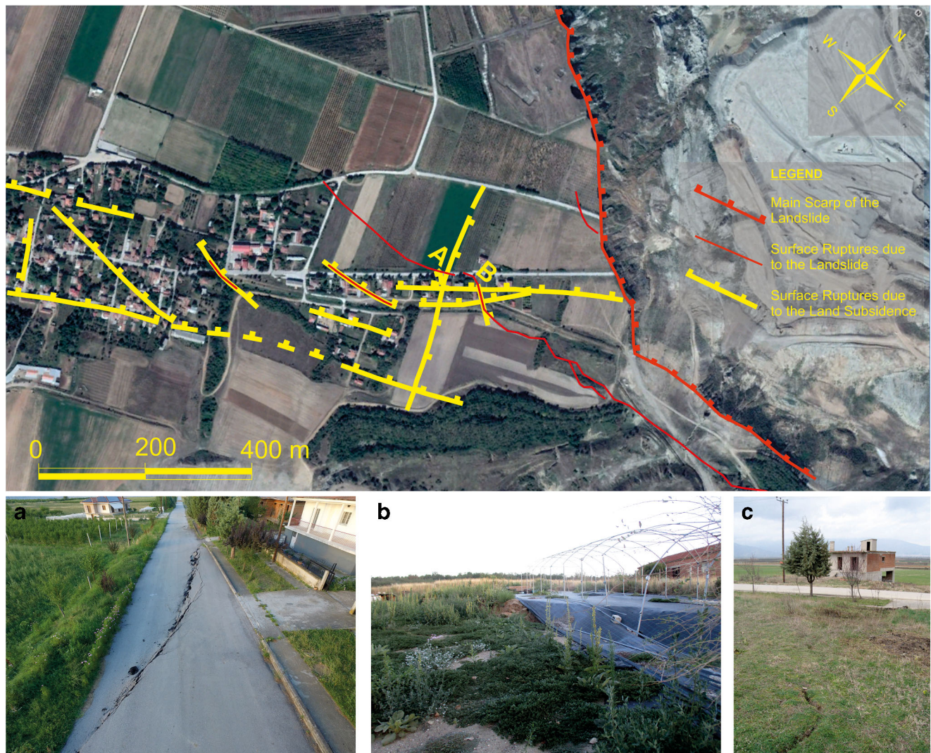
Fig. 11 The overlapping of the surface ruptures caused by the land subsidence phenomenon with those triggered by the landslide proves their interaction at the southwestern section of the working slopes. a , b
