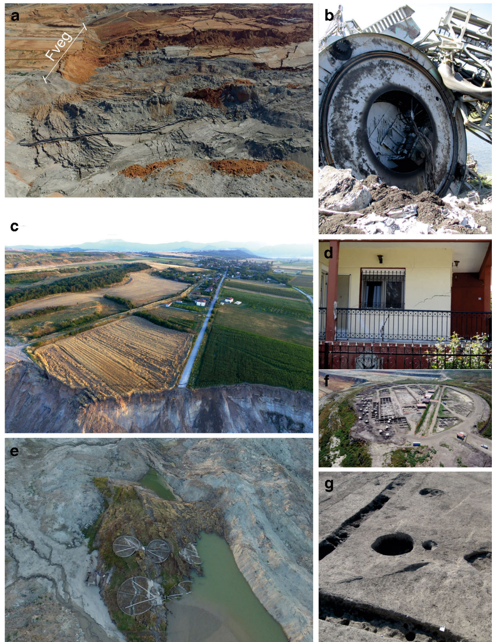
Fig. 7 a A closer view of the western boundary of the landslide. Several meters of destroyed conveyor can be identified. The part of the outline coinciding with a segment of the Vegoritida fault is clearly indicated. b A 1500-ton bucket wheel excavator buried by the landslide. c A view of the part of Anargiri village affected by the landslide. The destroyed road network is also clearly presented. d One of the houses in Anargiri village damaged by the landslide. e The wastewater treatment plant of Anargiri village collapsed inside the open cast. f One of the archeological sites of the lacustrine Neolithic settlements located at the perimeter of the open cast before the occurrence of the landslide. g A closer view of an archeological excavation. The preserved traces from the wooden piles used for the foundation of Neolithic houses are presented
